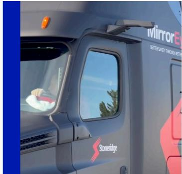
At FreightWorks our core commitments to safety and innovation are always about drivers' needs first and foremost.Recently we had an on-site demonstration of the incredibly innovative MirrorEye Camera Monitor System by Stoneridge. MirrorEye is a new solution designed to fully replace traditional mirrors on Class 8 trucks with a combination of wide angle cameras mounted outside the cab, and mirror-shaped screens mounted on the A-pillar inside the truck.
